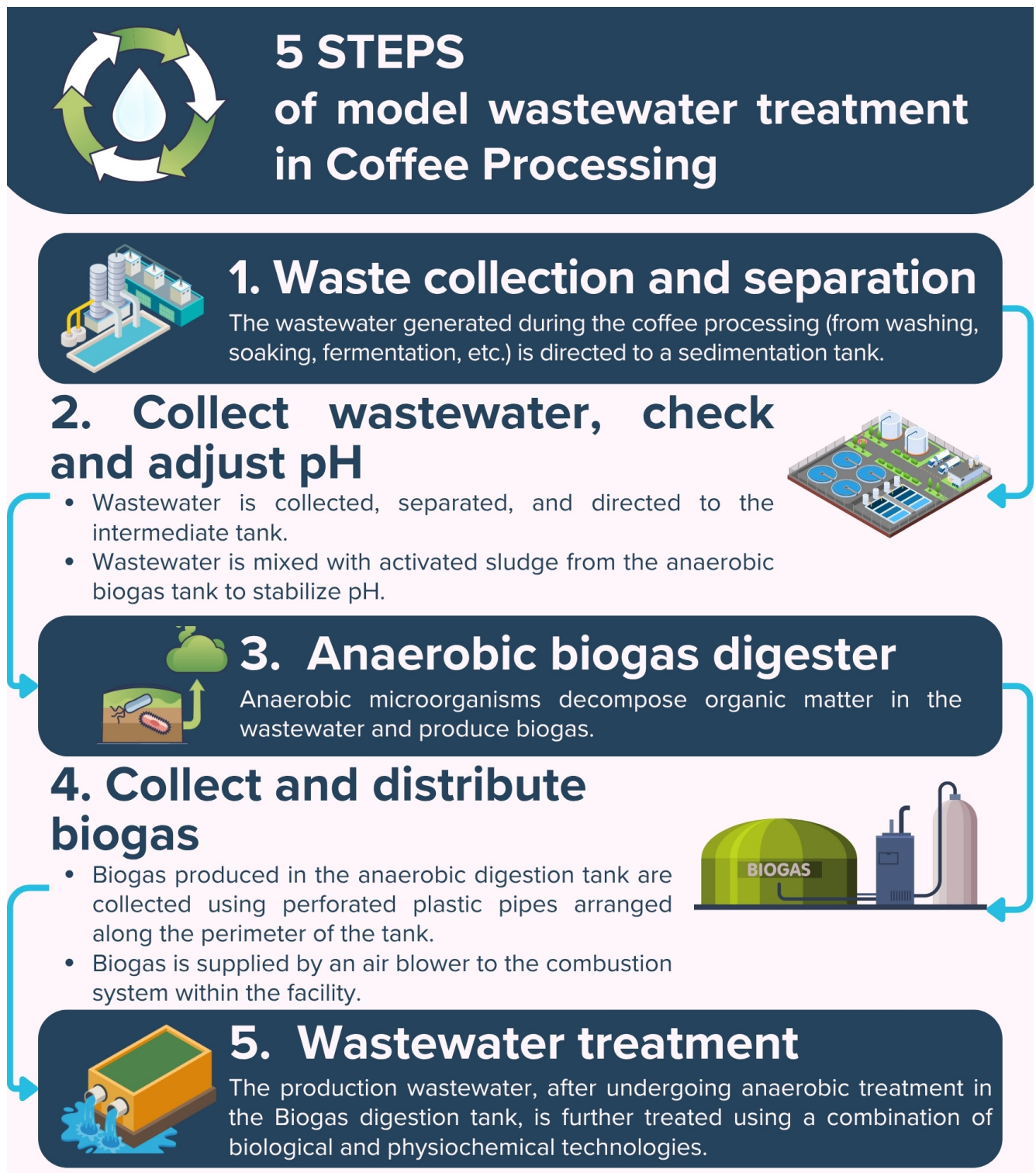
Figure 9. 5 steps for wastewater treatment in coffee processing
