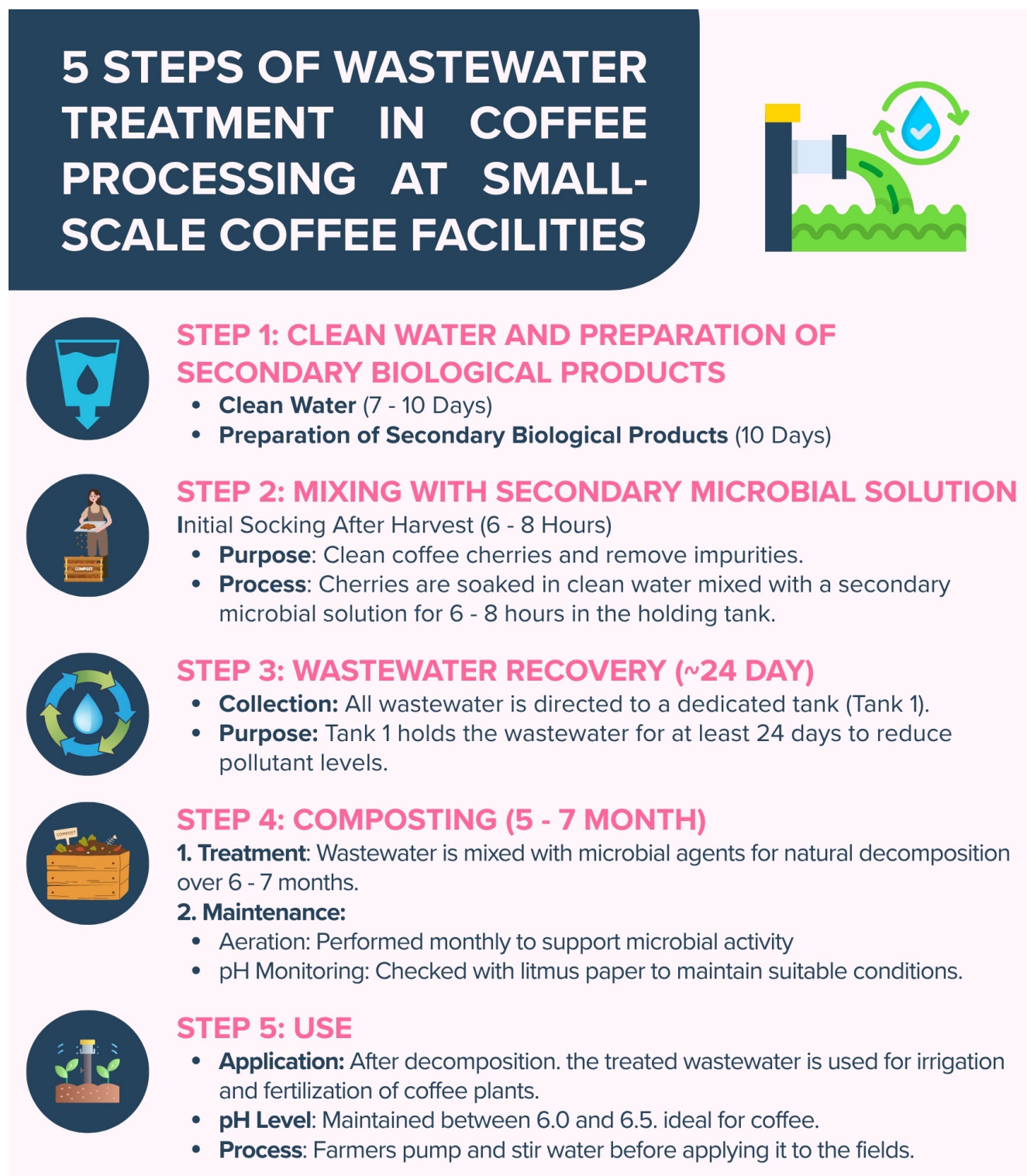
Figure 7. 5 steps of wastewater treatment in coffee processing at small-scale coffee facilities
